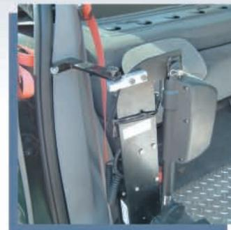
Bracket Secures Ramp to C-Pillar
